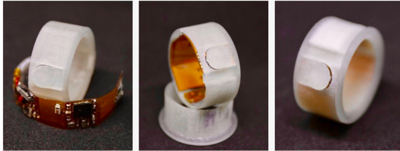
Fig. 6. Bluetooth wearable ring used to trigger the headset. The ring contains a custom-made FPCB with a micro switch and a Bluetooth Low Energy IC (Nrf51822)
