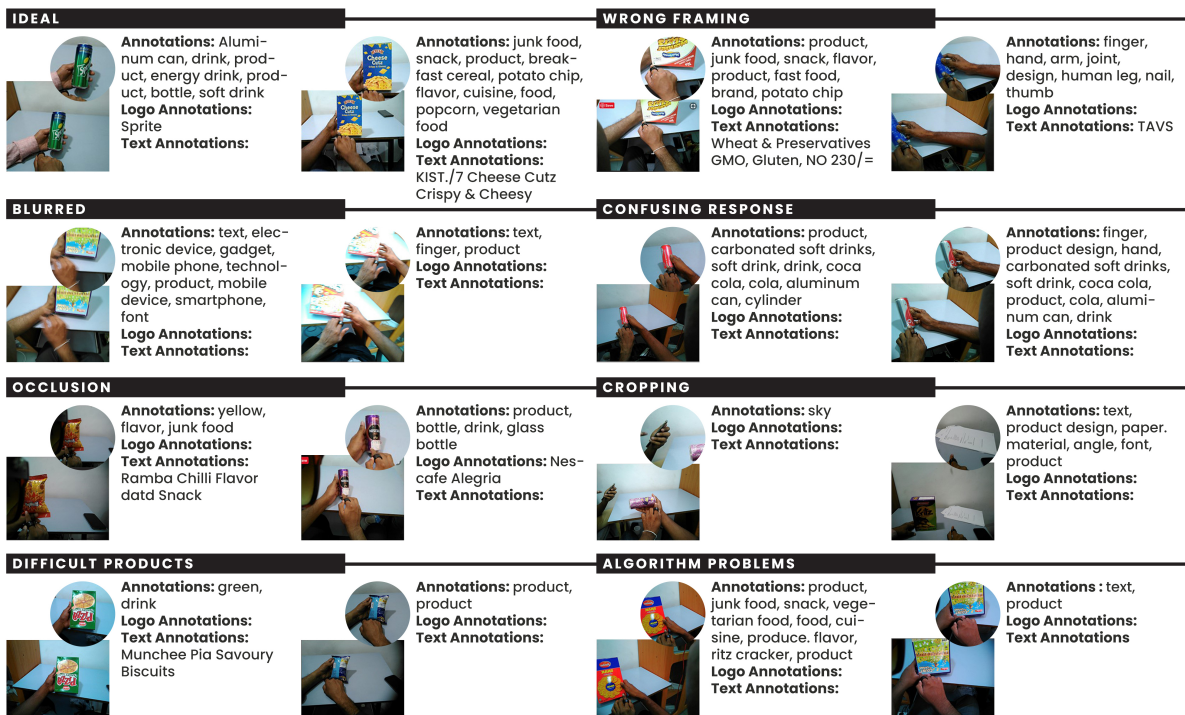
Fig. 8. Subset of images that show the different challenges faced to provide reliable feedback. Each of the instances contains its original picture and the ROI picture. Also, at the bottom of each image, there is the answer given by the algorithm before applying a filter.
